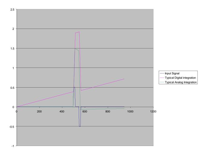
Digital integration also requires approximately 2X or greater bandwidth than an integrated signal as illustrated above. The rise time of the input signal is much faster than the risetime of the actual integrated signal.
