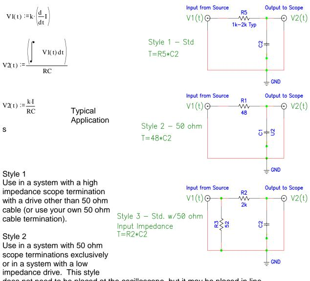
does not need to be placed at the oscilloscope, but it may be placed in line.
