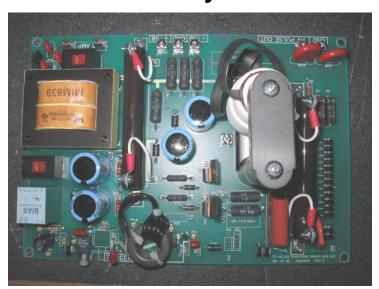
North Star High Voltage offers thyratron driver boards without chassis for general purpose use. These boards are generally combined by the user with reservoir and heater circuits to make a complete driver package. The board can then be mounted in the same enclosure with the other support circuits.
