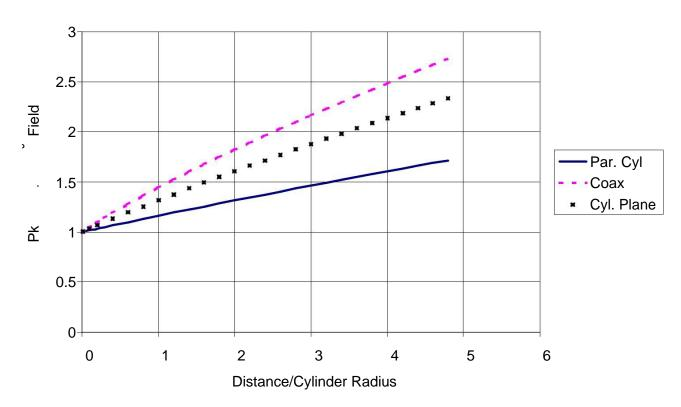
Field enhancement factor for cylindrical configurations. Upper: coaxial line, Intermediate: conducting cylinder adjacent to a plane. Lower: two parallel conducting cylinders
