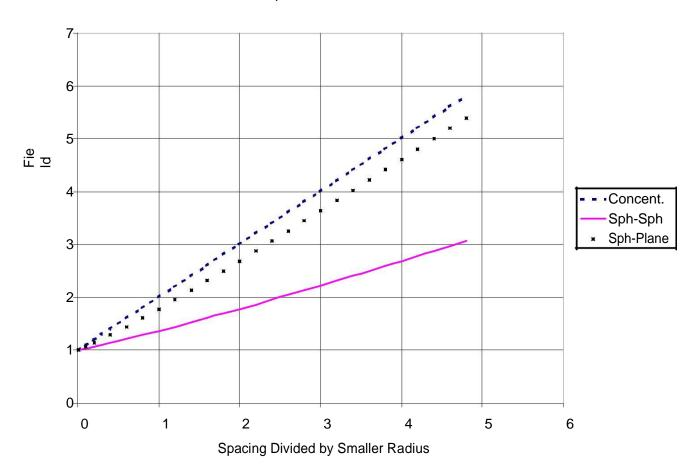
Spherical field enhancement including concentric spheres (upper) sphere-plane (middle) and adjacent spheres (lower).
