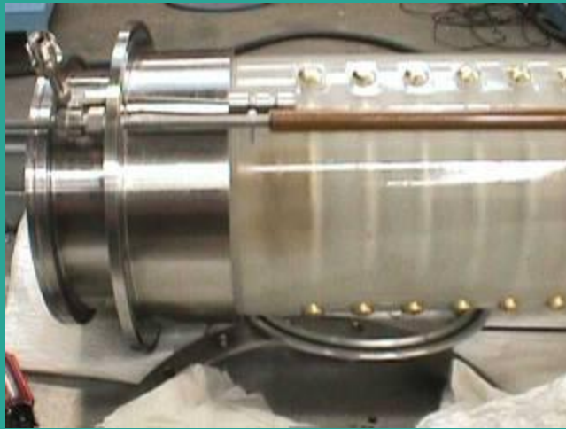
Vacuum accelerator column With some electron discoloration
