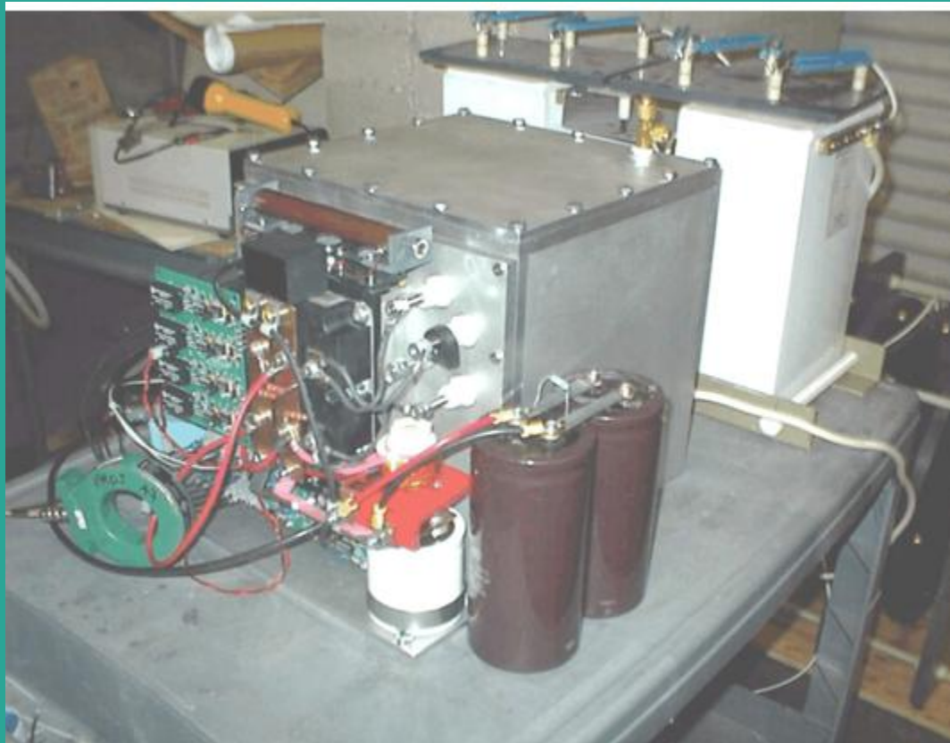
NORTH STAR 100 KV, 20 kJ/sec DC-DCHV POWER SUPPLY
