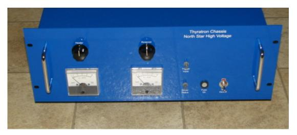
It is often convenient to purchase a unit which combines the thyratron driver, heater power supply, and reservoir power supply in a single unit. We provide a standard unit for this purpose as shown above.
