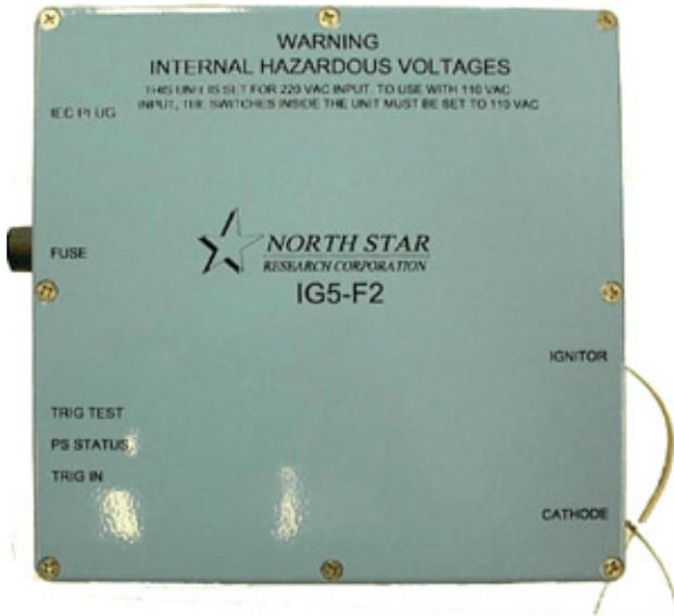
Ignitrons provide a unique high current switching capability for lasers, metal forming machinery, and a variety of capacitive discharge equipment. The IG5 unit meets or exceeds all ignitron requirements. It is delivered in a die cast aluminum box with convenient mounting studs. Only line power and a trigger are required for trigger pulse production.
